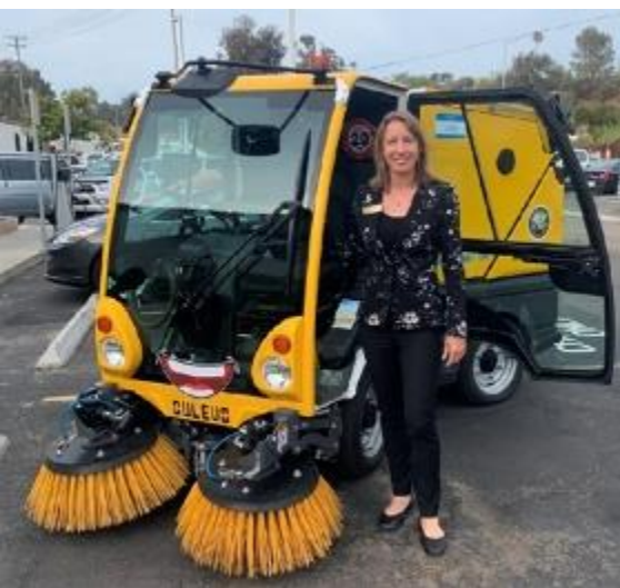
Figure 2. Example of special narrow street sweeper that had to be purchased to clean separated bikeways that were too narrow for standard street sweepers.
